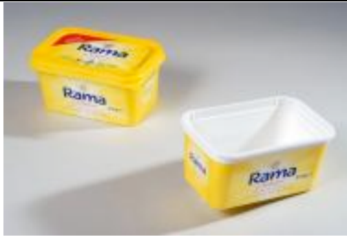
Picture 1. The Rama 500 g. margarine tub is produced using Veriplast's SLIM (Super Light Injection Molding) process, which relies on the MuCell® microcellular foaming process from Trexel for weight reduction without loss of quality in the molded tub.
