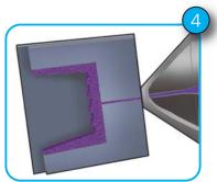
Low pressure filling of mold cavities. Pack & hold phase is replaced by controlled cell growth, which ceases once the mold cavity is filled. Cell growth results in a uniform pack pressure throughout the mold cavity.
