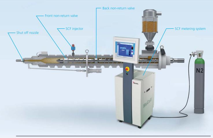
The technology can be easily integrated into new (OEM Model) or existing (MMU Model) molding machines:
