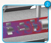
Homogeneous mixing and disbursing of the supercritical fluid into the polymer through the specially designed mixing section of the plasticizing barrel, creates a single phase solution of SCF and molten polymer.
