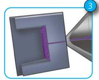
Injection of polymer into mold cavities. Cells start to nucleate once exposed to lower pressure in the mold cavity. Molecular dispersion of SCF provides for a homogeneous closed cell structure with a solid skin layer.
