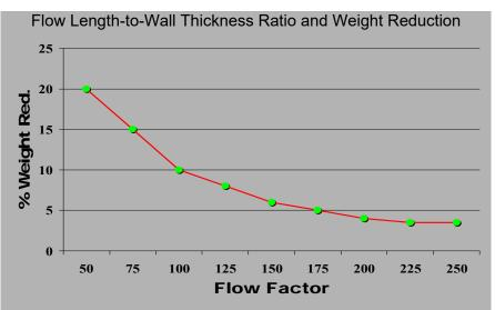
The dominant influence on weight reduction is the part's flow length-to-wall thickness ratio. This value places an inherent limit on the maximum weight reduction possible with the MuCell process.
